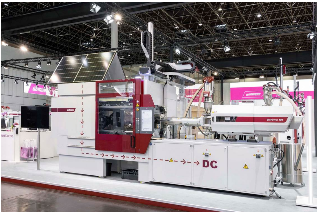
Fig. 2: EcoPower 180 DC – Concept study of an all-electric injection molding machine that can be operated with direct current
