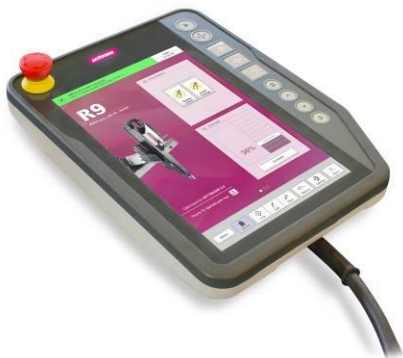
Fig. 3: WITTMANN R9 Teachbox – the display frame is injection-molded on a SmartPower 240
