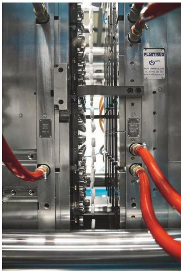
Fig. 3: Highly dynamic ejector for quickest demolding (photo: Plastisud)
